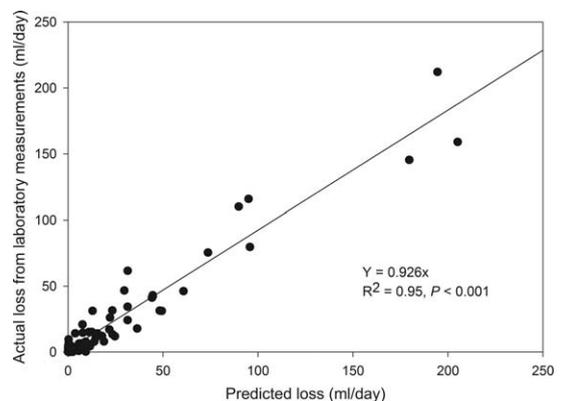
Fig. 2. Regression analysis of the predicted evaporation rates from the model (x-axis) and laboratory measured evaporation rates (y-axis). Resulting equation is actual evaporative loss =  $0.926 \times$  predicted loss. The 95% confidence interval for slope was between 0.868 and 0.983.
