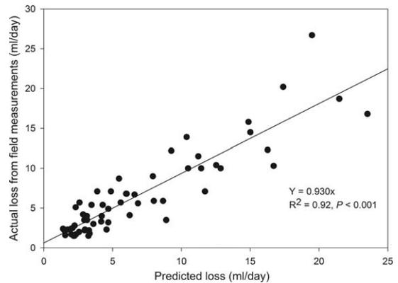
Fig. 1. Regression analysis of the predicted evaporation rates from the model (x-axis) and field measured evaporation rates (y-axis). Resulting equation is actual evaporative loss =  $0.930 \times$  predicted loss. The 95% confidence interval for slope was between 0.860 and 0.999.
